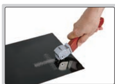
step 1: make grid cutting on surface
