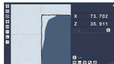
scanning the maximum profile of cutting tools
