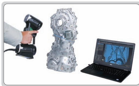
deep hole scanning: 1 blue laser line
