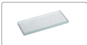
50mm reading scale (check magnification accuracy)
