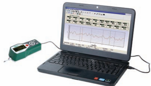
operate roughness tester by computers
