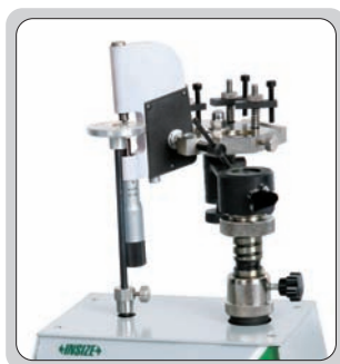
check the measuring force of indicating micrometers
