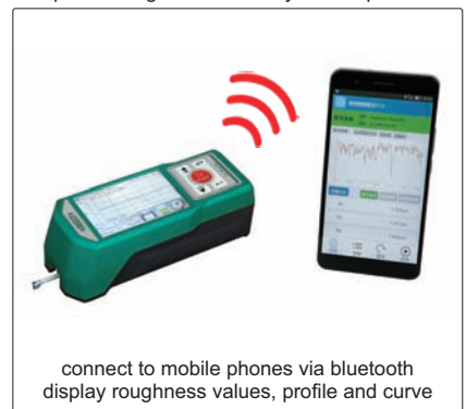
operate roughness tester by mobile phones
