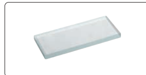
50mm reading scale (check magnification accuracy)
