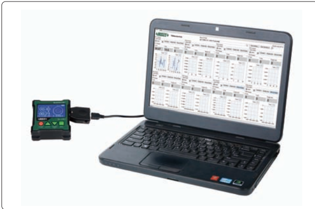
connect to computer via wired data transmission
