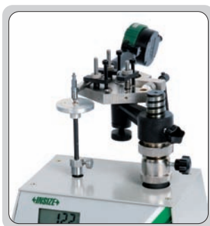
check the measuring force of bore gauges
