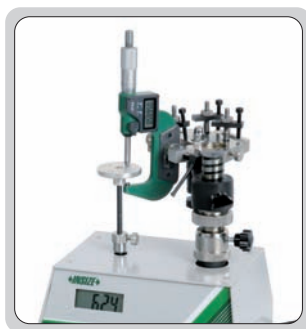
check the measuring force of micrometers
