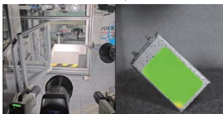
battery pack drop test strain field picture
