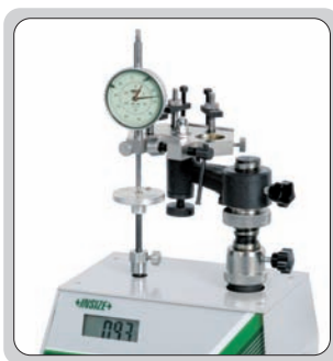
check the measuring force of dial indicators
