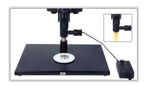
for smooth surfaces and small holes, brightness is adjustable
